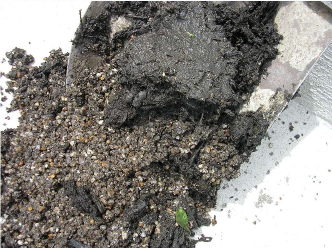
Figure 50. Study site B motor oil from oil service station caked on mulch surface in 2005
