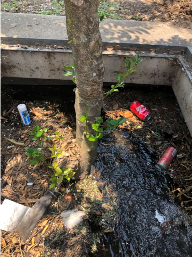
Figure 82. Initial flow during unsaturated test phase
