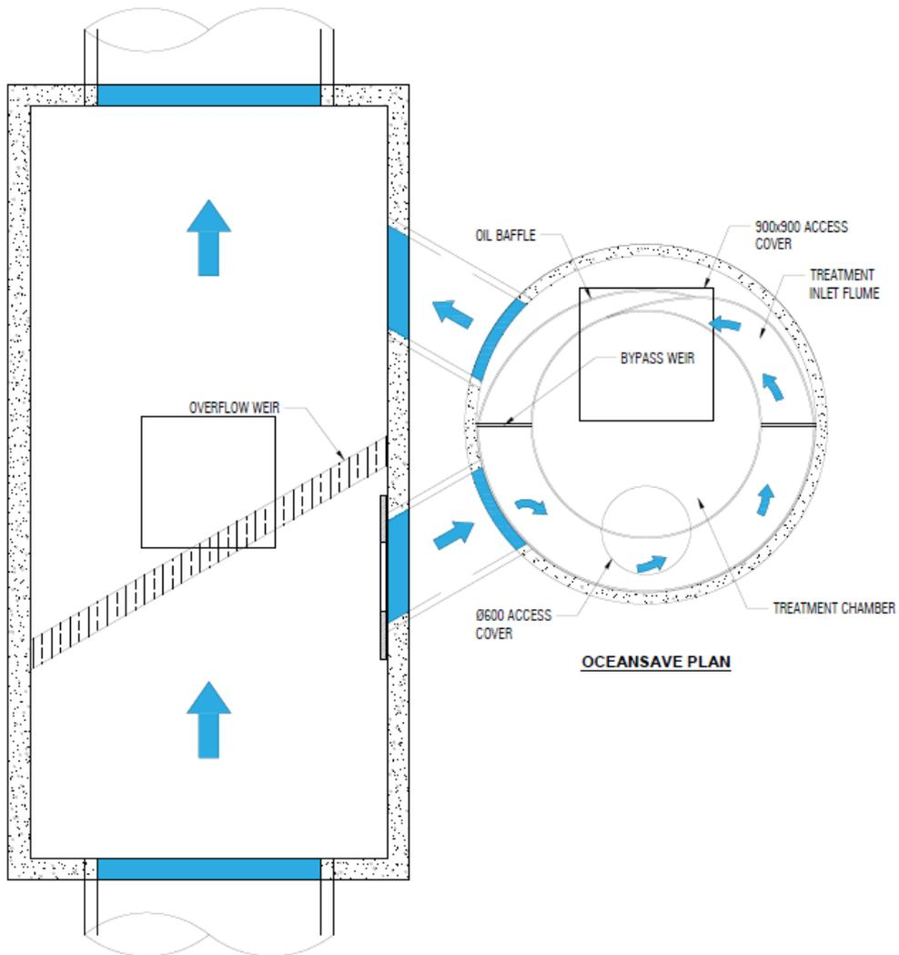
Figure 2. OceanSave-D Offline (typical)
