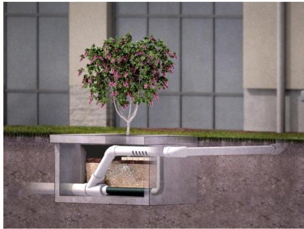
*Figure 5: Filterra tree pit – with internal bypass*
