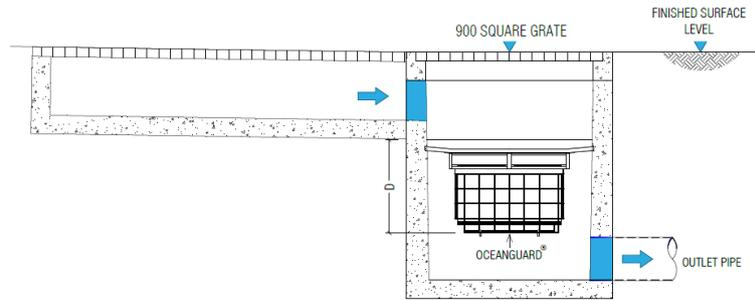
Figure 4: Example configuration – Grated strip/trench drain
