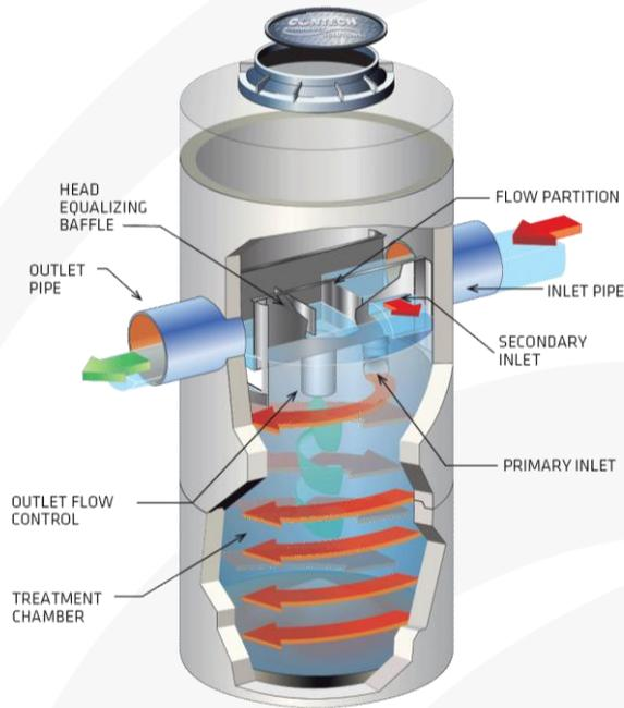
Treated stormwater exits the treatment chamber through the outlet flow control which helps maintain the helical flow patterns developed within the treatment chamber. A flow partition allows for stormwater to bypass during high flow conditions and the head equalising baffle reduces the potential for re-suspension or washout of captured pollutants during higher flow conditions.
